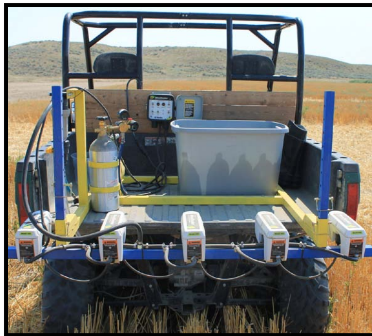
Figure 1. ATV-mounted sprayer fitted with LASC (Weed Seeker). 5 weed seeker units and a controller. Each unit fitted with 6702 nozzles with 12" spacing (5' boom). Height adjustments of 18 to 30". Equipment cost: 5 Weed Seeker units plus 1 controller: $8000. Photo by Prashant Jha, MSU-Southern Ag. Research Center, Huntley, MT, 2013.
